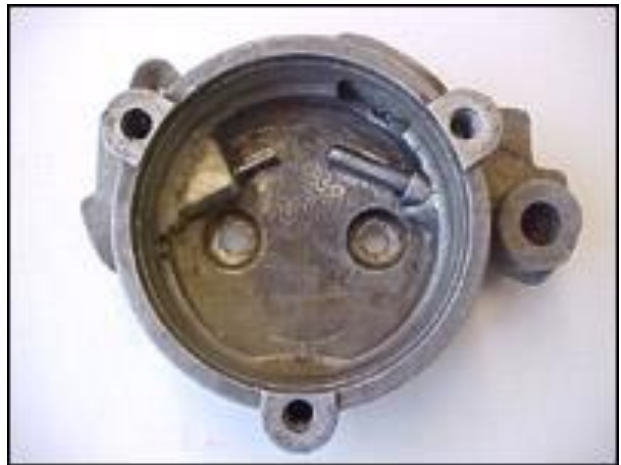
This is a '58 - '61 cold enrichment housing with the bakelite cover assembly removed. The piston on the left cuts off vacuum to the enrichment diaphragm when it is fully extended. The larger piston on the right sends a vacuum signal boost to the main diaphragm when it is depressed.
