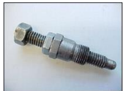
This is a Piston Stop Tool made from an old spark plug and hardware store nuts/bolts.
