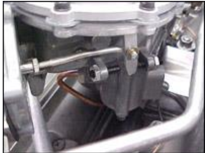
The blackened horizontal screw on the left is the Economy Stop; the screw on the right is the Power Stop.
