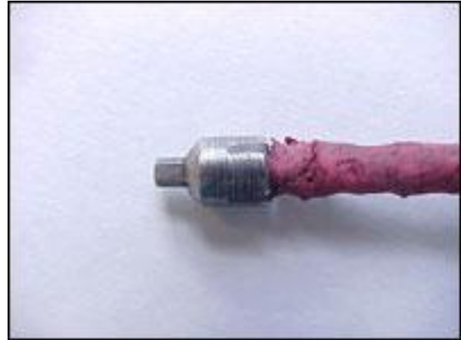
This is the tiny hex head tip of the Enrichment Stop Adjuster tool.
