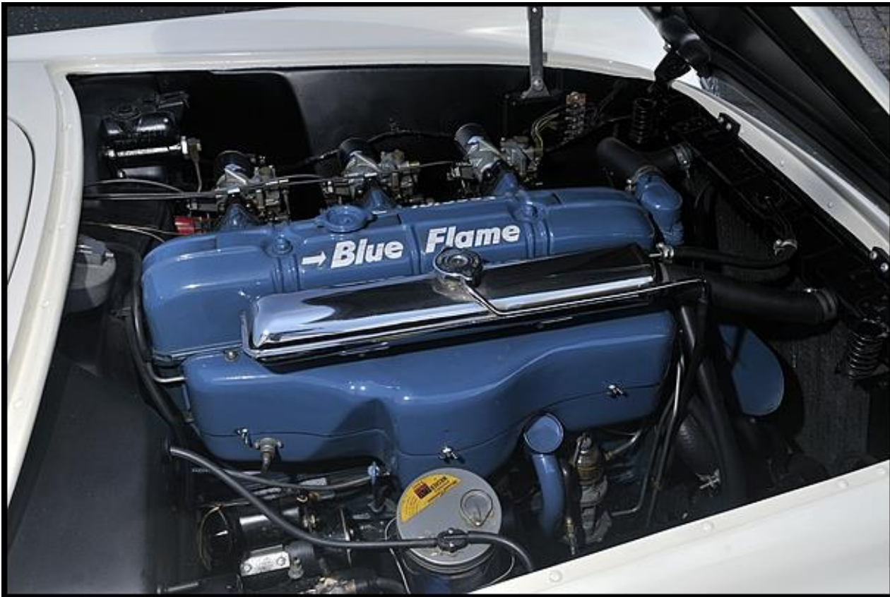
Via The Blue Flame Six was the first engine of the 1953 Chevy Corvette.
