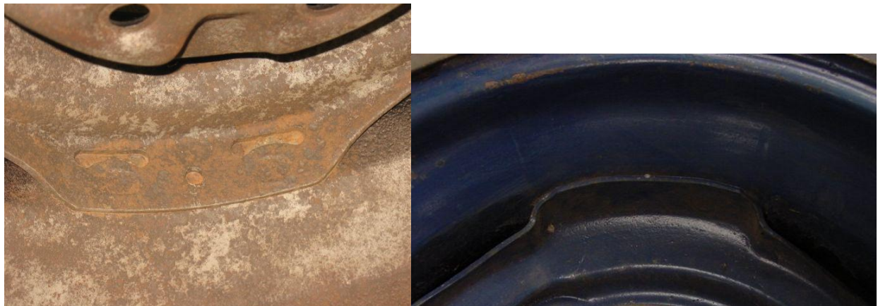
1955 – Mid 1959 > Dog-bone welded Mid 1959 – 1962 > resistance welded
