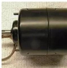
Heater Motor Rebuild Heater Motor Seized?
