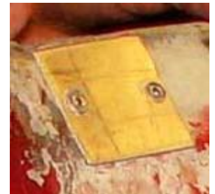
Taped on sheet metal covering existing old screw hole. 1/8" holes to the side are drilled through door and will house the pop rivets.
